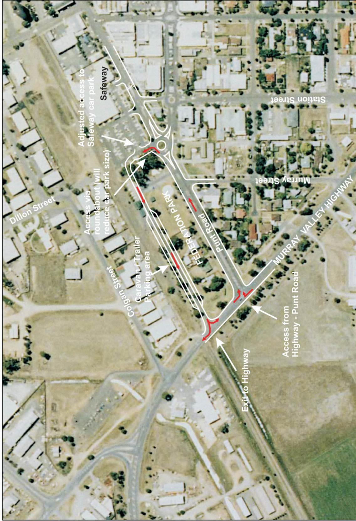
**CONCEPT C** - Draft sketch of possible access for caravans and car/trailers into a new long vehicle parking area and possible extension of Dillon Street.
