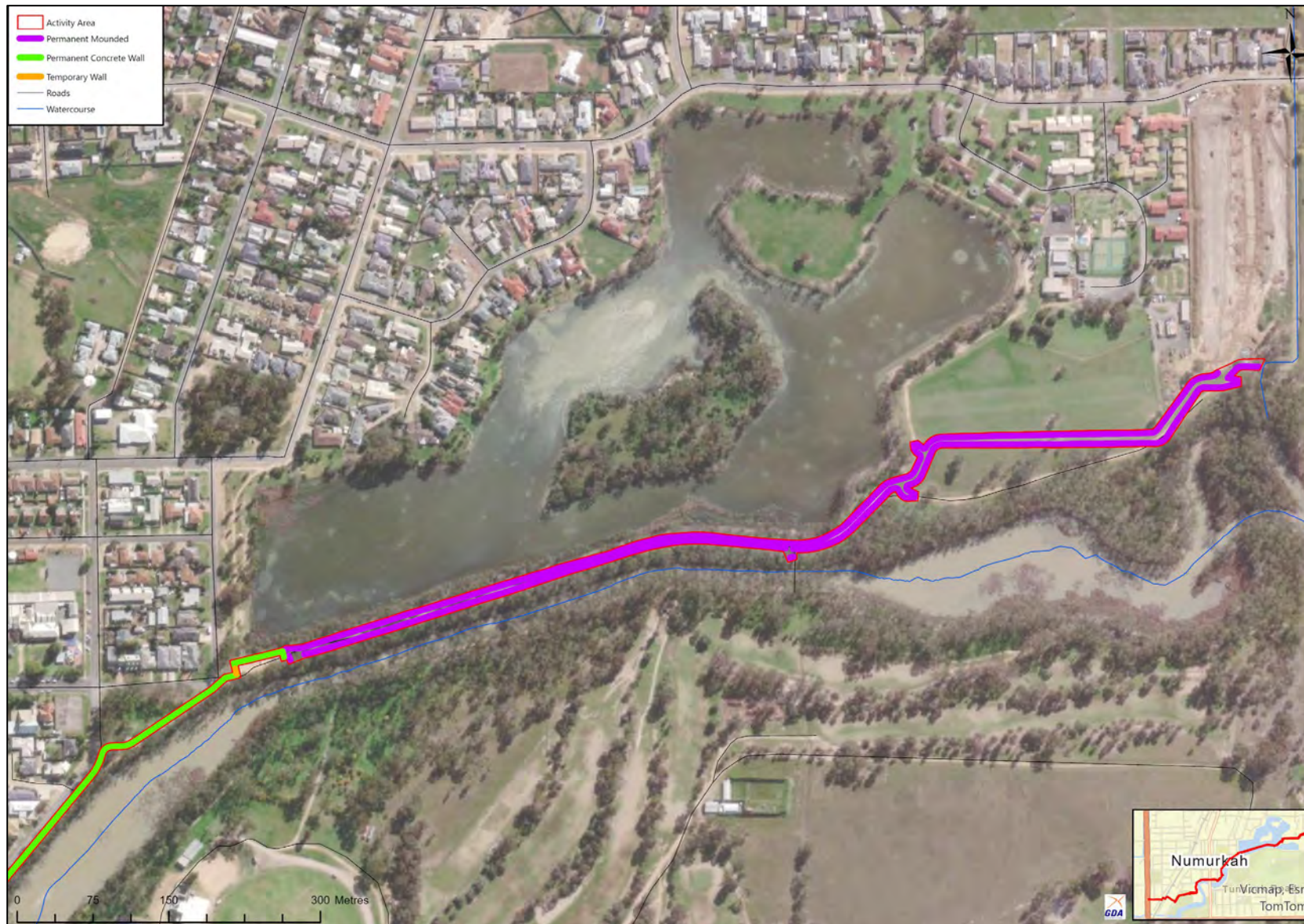
Map 2B: Proposed construction types of each section of the proposed levee. Source: Esri, 2024. Scale: 1:4,500
